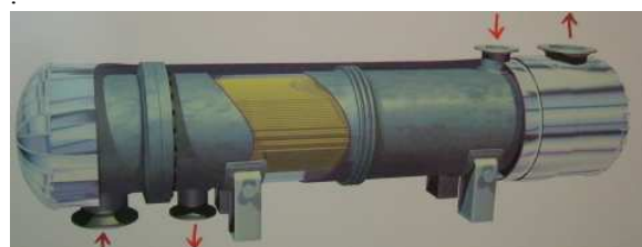
Fig. 2 Heating water heat exchanger at Nesjavellir
